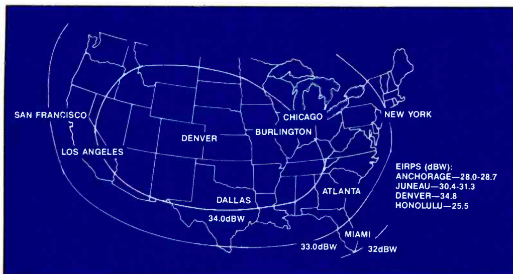
Figure 2. Effective isotropic radiated power (EIRP) is a measure of the relative strength of the satellite TV signal expressed in dBW. This footprint map graphically illustrates how strong the satellite signal is as it reaches various regions of the satellite's coverage area. Each satellite has a different coverage pattern. In many cases, different transponders on the same satellite will show a different EIRP. Where the signal is strongest is the area referred to as the boresight.
